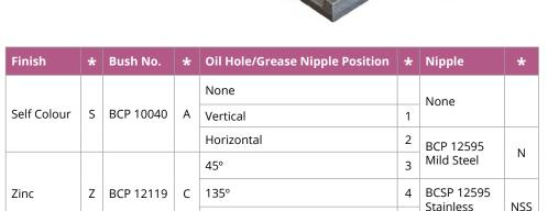
\*When ordering, please add the above 'characters' to the part number to indicate required condition, e.g. BCP10524DMSA1N indicates self colour with BCP10040 bush, vertical oil hole and BCP12595 mild steel grease nipple.
