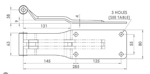
Model No. **BCP13607** (Mild Steel) Model No. **BCSP13607** (Stainless Steel) **Pressed Hinge 312mm**
