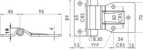
Model No. **BCP13302BOZ** (Mild Steel) Model No. BCSP13302-BOV (Stainless Steel)
