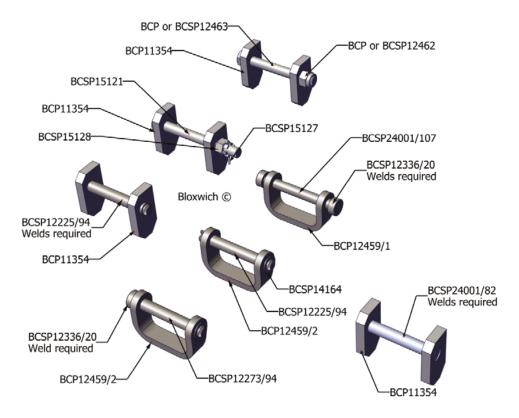
Model No. BCP1032-001 (Mild Steel) Model No. BCP1032-002 (Mild Steel) Model No. BCP1054-001 (Aluminium)
