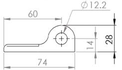
Model No. **BCP14149** (Mild Steel) Model No. BCSP14149 (Stainless Steel)
