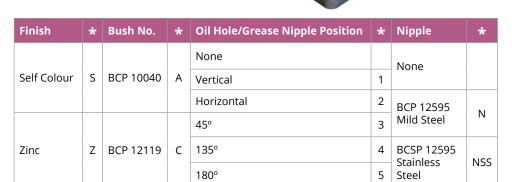
\*When ordering, please add the above 'characters' to the part number to indicate required condition, e.g. BCP11026SA1N indicates self colour with BCP10040 bush, vertical oil hole and BCP12595 mild steel grease nipple.
